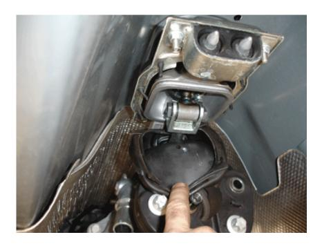
**Step 12**: Pull the underside rubber boot away from the shift body to reveal the shift selector arm connection. Similar to the front shift body legs, the selector arm is connected to the shift lever with a pin and two clips (one on either side). Using some long nose pliers, pull both clips off and remove the pin. The shifter should now be totally disconnected from the vehicle.
