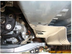
**Step 10**: Using a 15mm socket and ratchet, undo the 4 gearbox crossmember bolts around 3/4's of the way out. Using some support under the gear box (car jack works fine), remove all four bolts. Allow the gearbox to hang enough to gain as much access to the shift area as possible without allowing any cables or sensor looms to be strained (around the catalytic converter area, and rearside of the block there is several sensors/looms).
