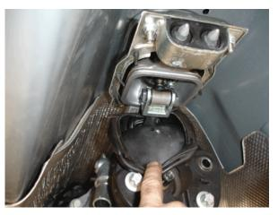
**Step 16**: With both clips removed from the selector arm connection pin, locate the selector arm on the shift lever and re-install the pin. Clip both retaining clips on to either side of the pin.
