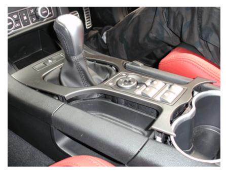
**Step 26**: It's a good idea now to take the vehicle for a test drive prior to re-installing the console surround to ensure the positive stop's are set accurately and to eliminate shaft vibration if the shaft is making contact with the stops.
