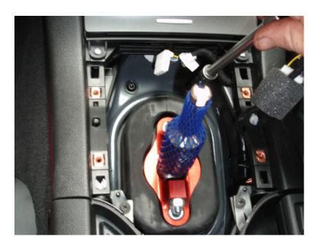
Step 22: Using the T-30 torx bit and driver, re-install the 4 shift body retaining screws to the vehicle body.
