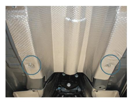
**Step 8**: Using a 10mm socket piece and ratchet, remove the exhaust heat shield.
