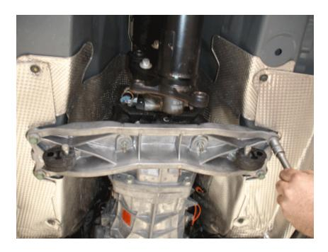
**Step 18**: Using a jack or person to assist, raise the gearbox/cross member back up to the vehicle, using a 15mm socket and ratchet, re-fit and tighten all 4 crossmember bolts. Be sure to check all bolts are securely installed.
