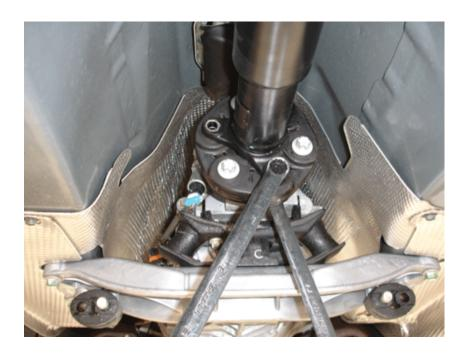
Step 19: Lift and slide the tailshaft back into position. Again, using 18mm and 19mm long handle ring spanners,
