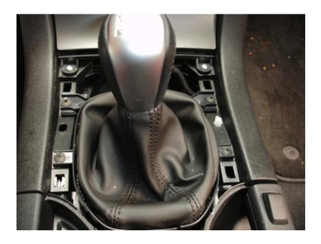
Step 3: Using a phillips head screw driver, undo the 4 retaining screws that hold the boot surround in place.
