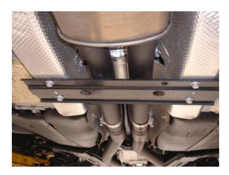
Step 21: Re-install black bracket to underbody using 15mm socket piece and ratchet.
