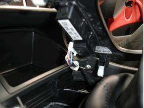
**Step 2**: Disconnect the traction control plug from under the front and the two rearward plugs for the power mirrors and window controls from beneath the interior console section. Once disconnected, remove the console section and place in a safe spot.
