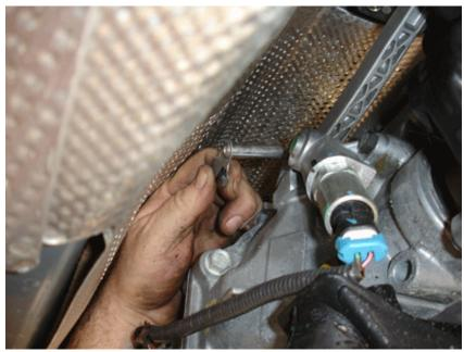
**Step 11**: On the top sides of the gearbox, you will note the two front legs of the shift body meet the gearbox and are retained by two pin's with slide clips. To remove these clips, you need to push the tab towards the center of the car and push the clips upwards to undo the lock. Once the clip is pointing upwards, simply pull each pin outwards to remove.
