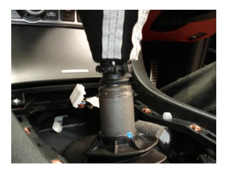
**Step 4**: Lift the boot up off the mounts, and carefully holding the gearknob only (do not hold/put force on gearboot surround or it may tear) firmly pull the gearknob off the standard gearstick. Once the gearknob and boot are removed together, place in a safe spot.
