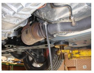
**Step 20**: With the 10mm socket piece and ratchet, re-fit the exhaust heat shield to underbody. Once the heat shield is in place, re-fit the center section of exhaust removed earlier in installation. Please ensure to re-clip in the o2 sensor looms near the catalytic converters.
