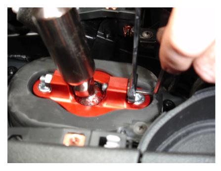
**Step 23**: With a 4mm allen key and 13mm spanner, adjust the positive stop's into position. To do this, it is best to adjust them in 3rd and 4th gears respectively. Selecting 4th gear, loosen off the 13mm nut on the positive stop and wind the stop to gently touch the shifter shaft. Back the stop off around 1mm or enough to not allow the shaft to rest on the stop, or to touch the stop under accelleration/backing off to prevent any potential vibration between the two surfaces.
