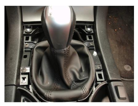
**Step 25**: Using a phillips head screw driver, re-fit and tighten the 4 gearboot retaining screws. Adjust the gear boot to sit neatly.
