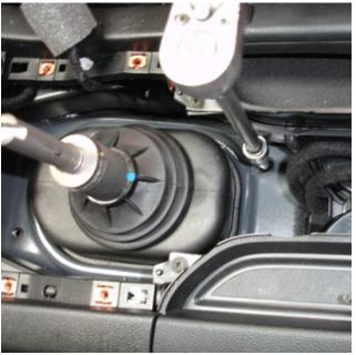
**Step 5**: Using a T-30 torx bit and driver, remove the 4 retaining screws for the shift body to the gearbox tunnel. Once all 4 screws are removed the shifter assembly will 'drop' down a little.
