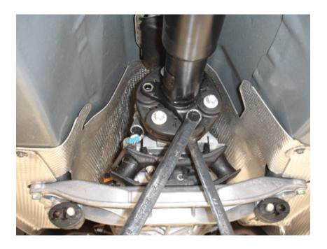
**Step 9**: Using 18mm and 19mm long handle ring spanners, undo the three tailshaft bolts in the rectangular pattern on the rearward side of the rubber join as pictured. Once undone, slide the tailshaft rearward slightly and support/let hang so as to create enough access to the shifter area.
