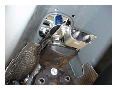
**Step 14**: Take your new Billet Pro series shifter, and as per the removal of the standard shifter, carefully manouver the assembly back into the same location. Once again, each car is different, but it can be a little tricky to get it in sometimes, but be patient.
