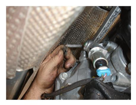
**Step 15**: With the shift assembly resting in place, re-insert the front two fork leg pins. be sure to push them dowards to clip back into the gearbox casing as per removal.
