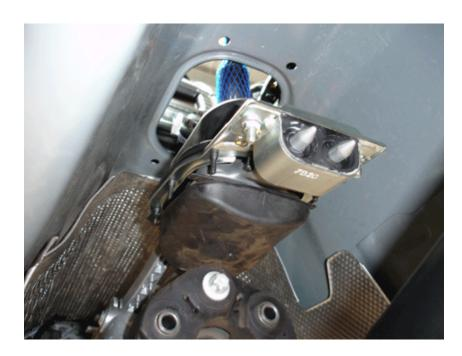
**Step 17**: Re-fit the factory selector arm boot to the groove located on the shift body as per OEM item.
