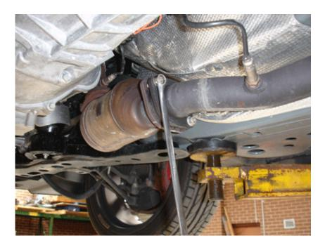
**Step 7**: From the catalytic converters, and just aft of the location of the black bracket you just removed, undo the exhaust system. Remove this section of the exhaust system and place aside. \*\*Exhaust pictured not standard item\*\*
