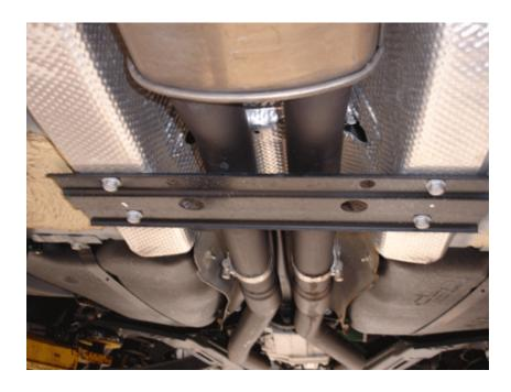
**Step 6**: Under the center section of the car you will note a black bracket below the exhaust system, this needs to be removed using a 15mm socket piece and ratchet.
