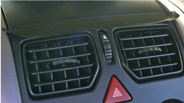
2) Using a flat tool such as a screwdriver, ease and pop off the original cover.
