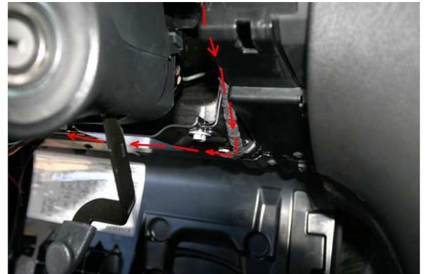
**15)** Attach the wires as shown on the picture. Black wire (ground) connects to the steering column bolt. It is highlighted blue on the picture. Connect the other three wires (white, red and pink) as shown on the picture insert: first, plug the wire into the right side of the fuse connector, then plug the fuse on top.
