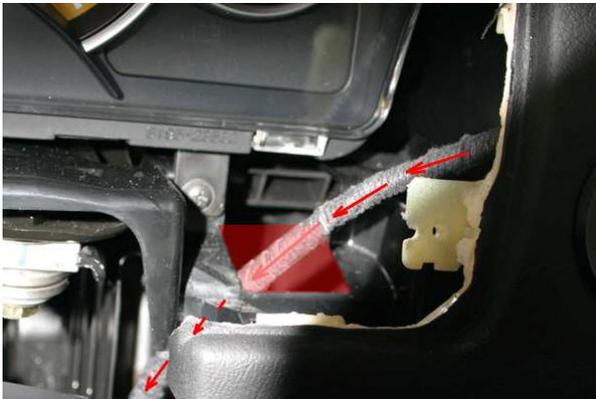
14) Route the wire underneath the steering column. You can use zip-ties to hold it in place at your discretion.
