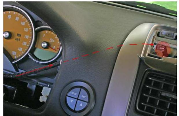
11) Cut along the red line. This allows for perfect fitment. **NOTE: THIS MUST BE CUT OUT. IF YOU DON'T, YOU RISK DAMAGING THE COVER AND/OR THE GAUGE MOUNT POINTS WHEN YOU CLIP IT DOWN.**
