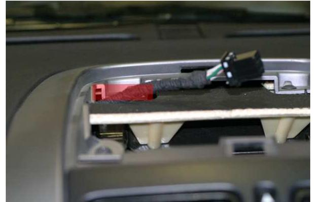
13) The other end of the wire harness should be pushed down through the opening as shown.
