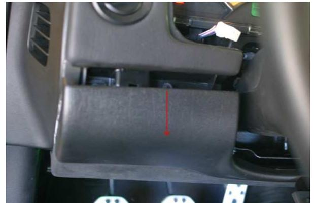
9) Take the wire harness and push the connector side through as indicated by the arrow.
