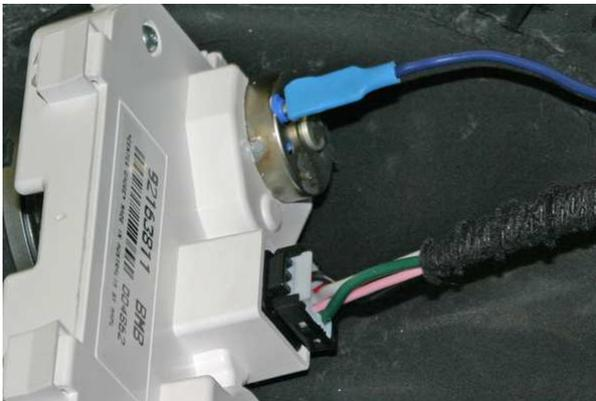
**18)** Clip the gauge in and peel the tape off.
