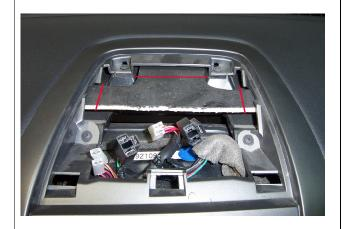
**8)** The plug for the gauges as seen below is taped to the wiring harness behind the climate control.
