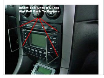
2) Metra GTO Radio Removal Tools \$11 From Installer.com. Notice how the ends are flared. This makes them able to remove the radio.
